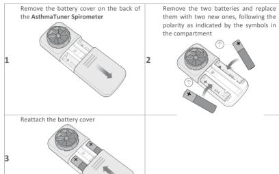
Used AsthmaTuner Spirometer batteries should only be disposed of in special containers or preferably returned to the dealer of the device or to a special collection centre. In any case, all applicable local regulations must be complied with.
